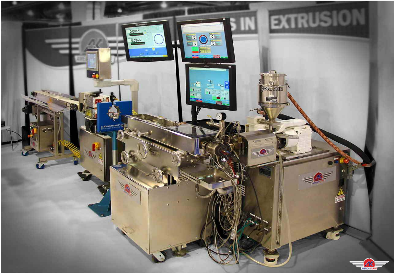
On display at Graham is an American Kuhne brand three-layer line for medical tubing.
